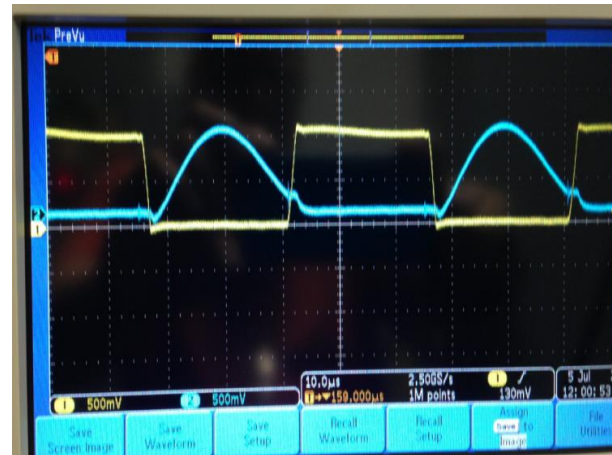
AT-HVCM IGBT Q1 V_{CE} (gold) and I_C (cyan) ZVS @ turn-on from magnetizing current
